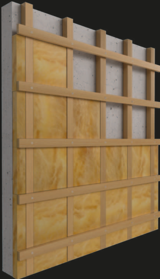
Installation of the substructure (sub structure) and the sound absorbing wool (insulation wool)
